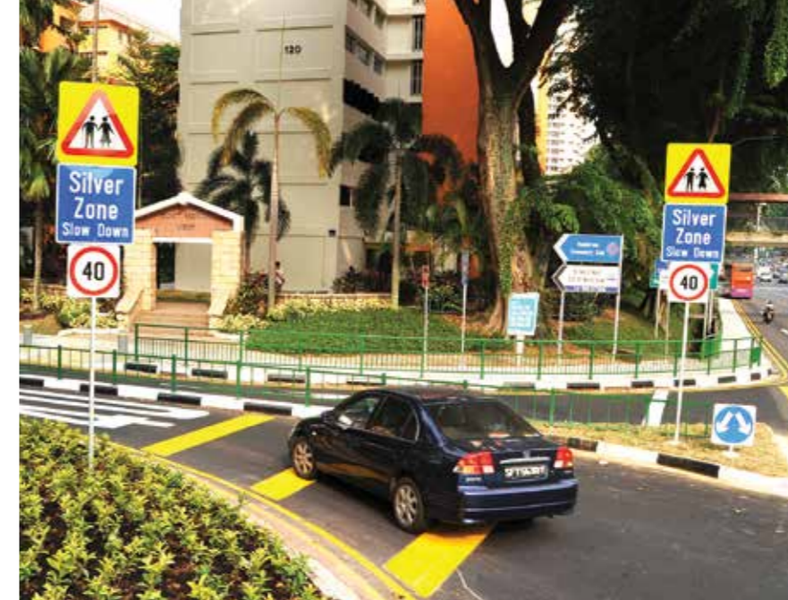
(Above) Silver Zone Gateway at with 40km/h speed limit and yellow rumble strips to alert motorists to slow down.
